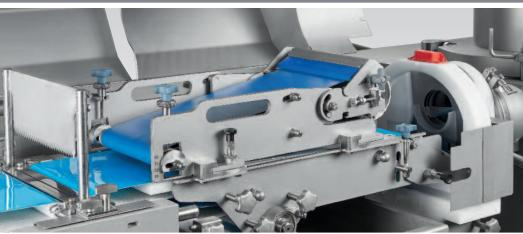
The continuous filling and cutting concept (without start - stop portioning action) enables the RS 920 Flex to be extremely fast and accurate compared to other systems on the market. This continuous working principle maintains aconstant and regular flow of product, increasing the production speed of minced meat portions, up to 200 PPM for mince and up to 250 PPM for burgers, whilst preserving the product texture and appearance.
